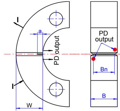
Figure 2. CS(T) Specimen.
